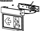
Snap AC supply on PCBA and then snap fixture to mounting plate.
