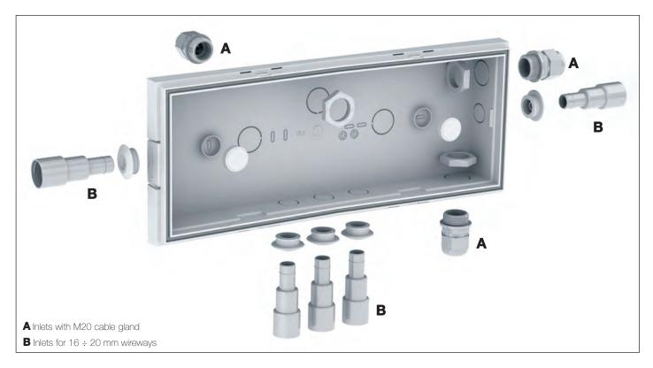
The mechanics of the lamp body has been studied in collaboration with a team of installers who have tested its versatility. Power supply inlets provided on every side, suitable for any type of wireway (16-20mm) or direct cable (M20 cable gland). The opening system has 4 snap hooks that allow access to the reflector and to the lamp circuit for wiring and manual adjustments (when not using the CableCom Connect APP)
