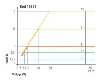
The output power is subordinated to the maximum out-put current of 500mA (e.g., with the inverter set to 1h of autonomy, it will guarantee a 7W output when only used to power an LED set with Vled>14Volt; below this voltage, the power is reduced as shown in the graph.
